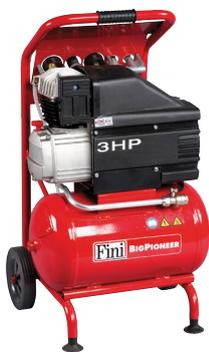
**Fini Big Pioneer** Fitted with a powerful 3 hp motor delivering 10 cfm [17 m<sup>3</sup>/h]. The large 20 L receiving tank is suited for small workshops or for paint frame use. This compressor is still very compact and portable although it is a bit of a heavy lift to get into a car. A 9 mm SATA-type hose will push fit directly to the compressor's connector. If you need to use 8 mm bore hoses see the Pioneer converter [page 75].
