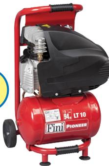
**Fini Pioneer 265M** This Fini compressor with a 2 hp motor delivers 7.6 cfm [15 m<sup>3</sup>/h] making it ideal for the freelance scenic artist needing a compressor which is easy to transport in the boot of a car. It takes a 9 mm SATA-type hose which will push-fit direct to the compressor's connector. If you need to use 8 mm bore hoses see the Pioneer converter on page 75.
