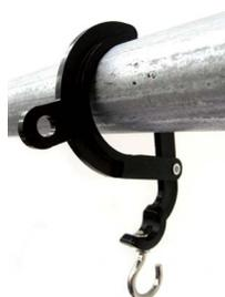
**Pipesnaps** A great product to radically speed up rigging and demounting drapes. The Pipesnap quickly clips onto any 50 mm Ø barrel. The weight of the cloth holds it securely in place. To release it, a cord can be attached to the hole on the rear of the clip. When the cord is pulled the clip cants back and releases from the bar. The clips can be linked with a cord so that fewer hauling cords are needed to release entire cloths.
