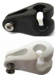
**Gauze Hanks** A very useful clip for fixing gauzes to tension wires. The clip grips the cloth by means of a small screw. The clip is then offered up to the tension wire at right angles and twisted to lock in place. The gauze can then silently slide up and down the wires whilst remaining stretched. Available in black and white. Also see Pelican Hooks [page 169].
