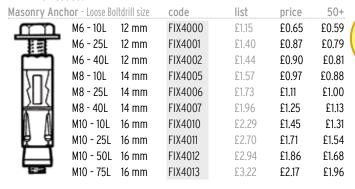
Masonry Anchors - Projecting Stud For fixings where a studding fixing is required, ideal for overhead work. Once fixed, the nut can be removed to release the object being held. For fixing trunking, wall plates, metal work, timber and structural fixings. When ordering Projecting Studs please note that the bolt size is given first, then the maximum fixing thickness [e.g. M6-10P has an M6 bolt and will hold down material no more than 10 mm thick].
