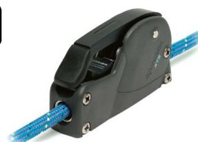
**Spinlock Powerclutch XTS** Spinlock are the experts in rope handling. Their position in the market is such that many countries refer to all rope clutches as "Spinlocks". The XTS rope clutch can handle ropes up to 14 mm in diameter. The ropes can be pulled through in one direction while the clutch remains engaged. To release, just lift the lever and the rope will run freely in both directions. For use with braided ropes [not three-strand or wire ropes] from 8 - 14 mm. Fixings: Ø M8 csk heads.
