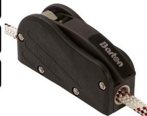
**Barton DO 550 Rope Clutches** Designed to offer a holding power of up to 550 kg and to control braided ropes up to 12 mm diameter. It requires little effort to use the clutches thanks to the ergonomically-designed handle and bolt-together construction, which also allows for ease of servicing.
