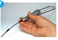
Remove your first tape marker (if used) before pushing the wire fully home in one even stroke until it reaches your second mark.
