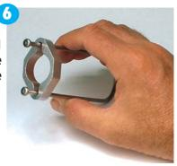
Now carefully insert the clean cut end of the cable 6mm into the "pilot cup" which is at the narrow end of the body. Ensure that the cable and deadend are free from grease or contaminates as this could cause failure.
