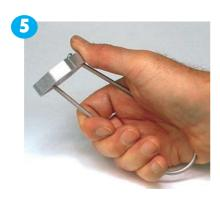
When they are together, as shown, they will slide over the main body. You will need to do this at this stage if the other end of the cable is already terminated or fixed off.
