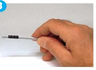
A second mark can be made anywhere along the cable so long as the wire has fully passed through the jaw mechanism.
