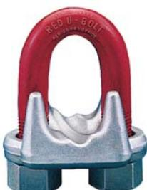
**Wire Rope Grips - Dogs** Notes Provides a simple and effective means of making a loop or a thimble eye in wire rope. Consists of U bolt, bridge and two hex nuts. The U bolt should be fitted over the non load bearing [short] tail of the loop, the bridge over the load bearing longer part. [Remembered by the mnemonic "Never saddle a dead horse"]. The hex nuts should be tightened equally, using a nutspinner or a torque wrench. For heavier loads use grips to DIN1142 or Crosby Grips.
