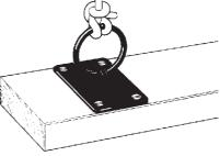
Ring Plates may be positioned at any strong point on the scenery. If the pull is not vertical then the Ring Plate should be aligned so that the pull is along the axis of the hoop which secures the ring.
