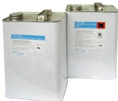
**Two-Part Polyurethane Foam Flame Retardant Formula [BS 4735:1974]** Flints supplies the latest HCFC-free system. The mix ratio is 1:1 by volume but the ISO component should be added to the RES component. The best way to mix is with a Paint Mixer on a drill [page
