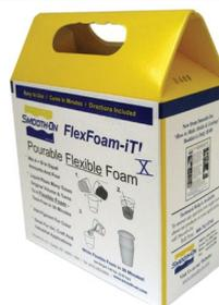
**FlexFoam-IT! X** A two-part soft foam with a very fine cell structure ideally suited for soft costume props. Simply mix part A and part B in equal quantities by volume and pour into the lowest point in your mould. The mould should have been treated with a non-silicone Release Agent [page 106]. It will expand to approximately 6 times the original volume and is tack-free in 30 minutes. Demould in 2 hours. Pot life is 50 seconds. Supplied complete with full instructions.
