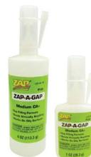
**Zap a Gap** Fills Gaps. Allows 7 – 10 seconds for positioning and cures in 20 seconds. Can be accelerated by using the aerosol [Kicker]. Bonds most materials including metal, wood, rubber, pottery, and most plastics. The aerosol [Kicker] is an accelerator only, not an adhesive!
