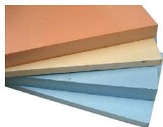
**Modelfoam** Fine-cell extruded polystyrene which is very easy to shape and form using conventional hand tools. It can be glued with Modelfoam Adhesive. Modelfoam comes in two grades – use the dense grade for finer
